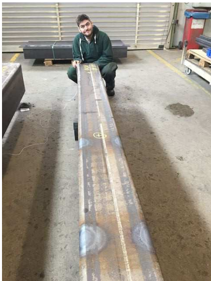
P5: The component having a plurality of heating bodies by flame
