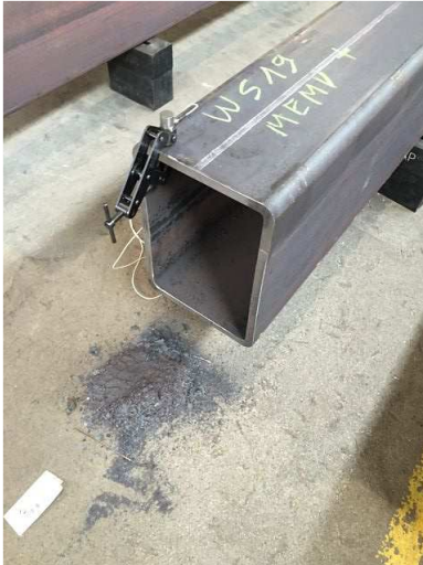
P6: The component loses scale by WIAP® MEMV® process
