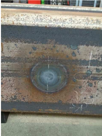
P3: flame straightening point
