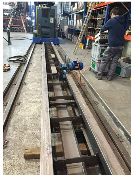
P9: machine stand during relaxation process. This was also directed flame
