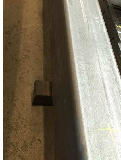
P8: Very important is a good rubber underlay. This should have a sufficient height so that no vibrations are transmitted in a factory building. In addition, the logging is accurate.
