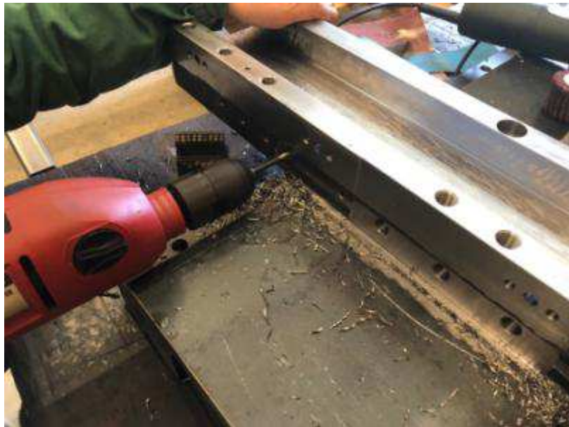
Deep hole drilling with hand machine.
