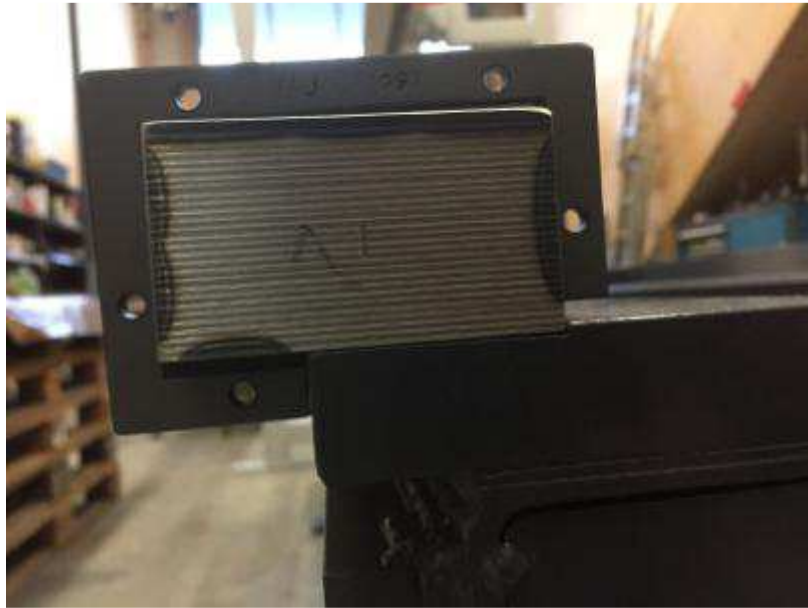
Figure 38 Scraper Specially made for WIAP 40x70 purchased for 3 machines in stock
