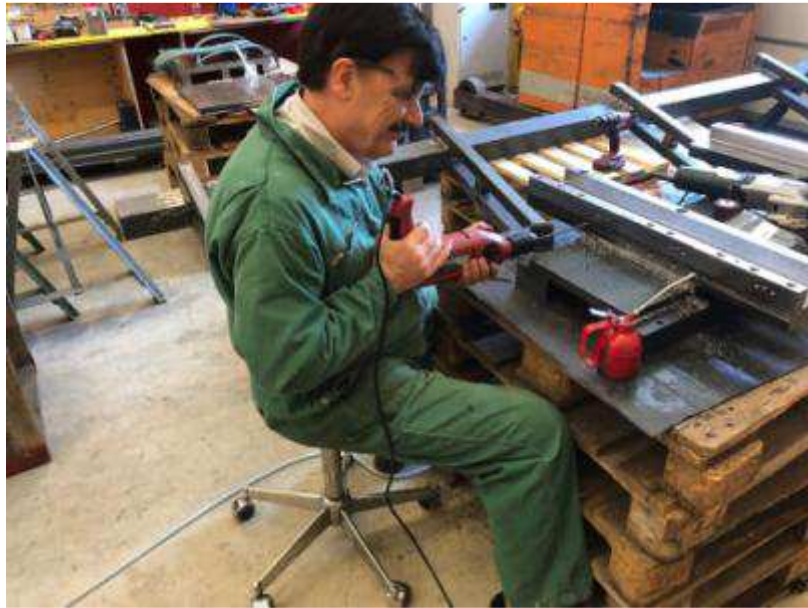
Deep hole drilling with hand machine.
