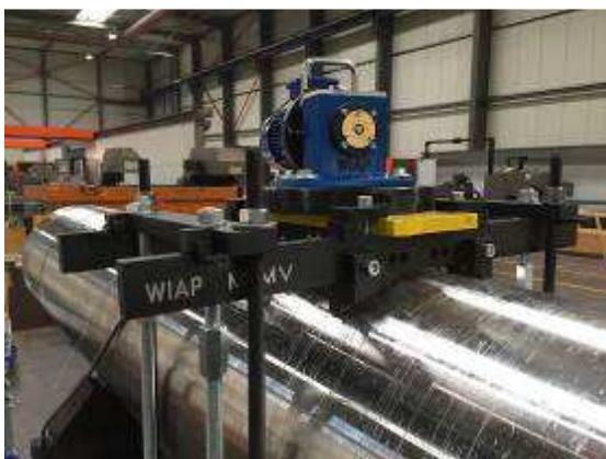
Figure 9b: rollers -Aufspannvorrichtung - robust connected to the component
