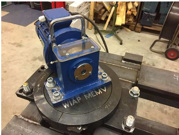
Figure 4: The CNC multi-functional machine bed WIAP DM3S at a vertical MEMV® treatment
