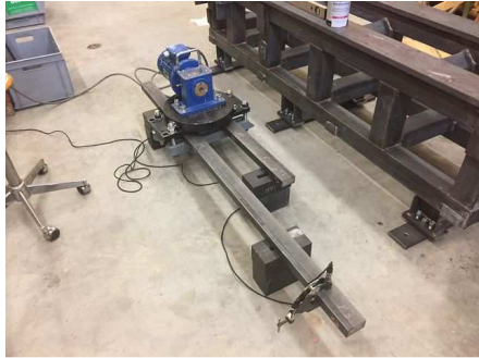
Figure 6: The "90 ° vertical WIAP MEMVrelax ® excitation is "transverse vibration modes
