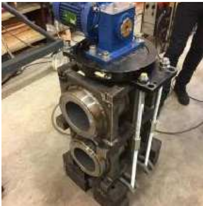
Figure 1: Two headstocks are vertically with the multi-function machine WIAP DM3S with the MEMV® (Metal relax with vibration) process relaxed (all photos: Hans-Peter Widmer)
