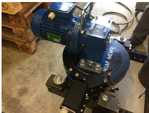
Figure 11: multi-directional WIAP vertical MEMV® machine with V 20 Stimulator
