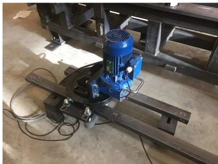
Figure 7: Horizontal WIAP MEMV ® relax: Horizontal and transversal waves are excited longitudinally generated. For thin components rotationssymmetrischen this Aufspannungsmethode is needed circumferentiale to produce excitation.
