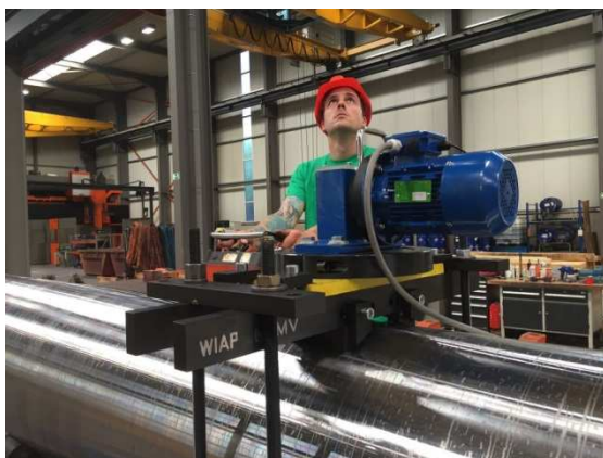
Rolls during vibration stress relief on metal (MEMV) - Jim Peter Widmer - April 2017 (hpw)
