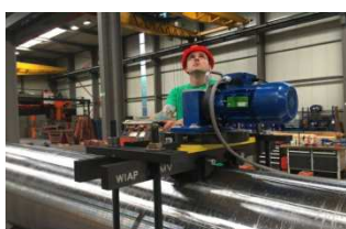
Fig. 5. Rolls during vibration stress relief on metal (MEMV) - Jim Peter Widmer - April 2017 (hpw)
