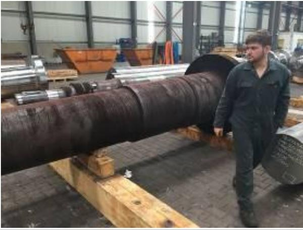
Figure 1: This 12000 KG roll-tension annealing requires 935 KW / H
