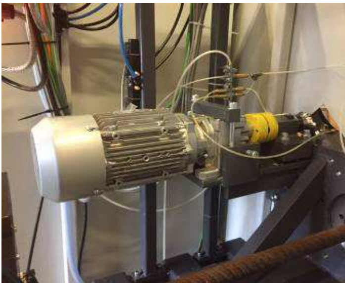
Picture 98: Food drive for 180 Nm. All diameters without jaw change possible. Lining can be freely opened enough to drive without interference contour with the loader to feed from behind. The lubrication lines are now installed throughout clean. The feed as the drive is everything lubricated automatically
