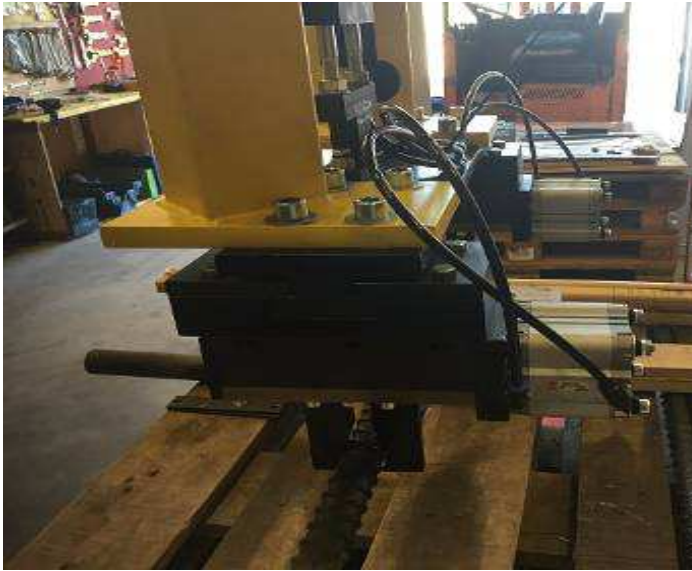
Picture 41: 2 grippers for 40 kg. It could be lifted safely even 80 kg
