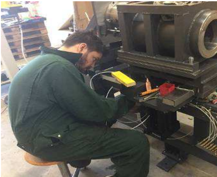
Picture 46: Sven, assembly of the lubrication
