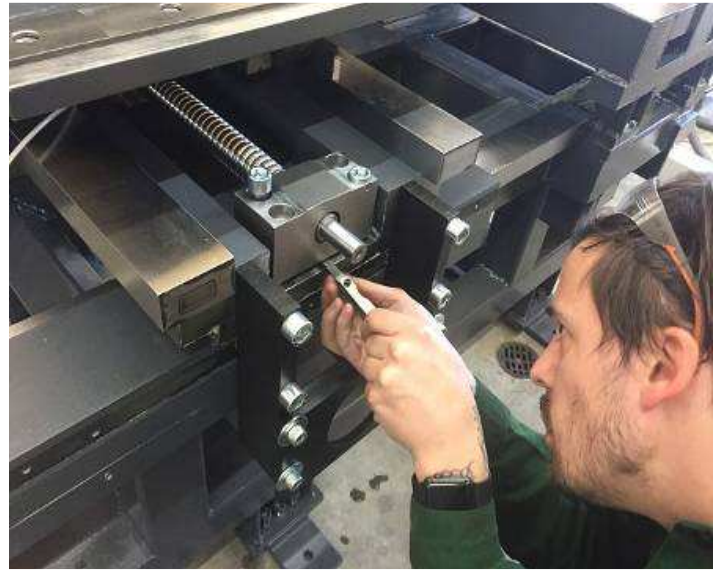
Picture 47: Jim, installation of X spindle
