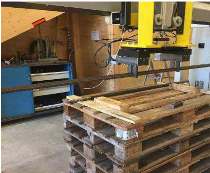
Picture 42: Test of the gripper with the HLV (auxiliary charging device)
