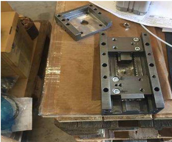
Picture 37: Parallel gripper 2 pcs. WIAP own design
