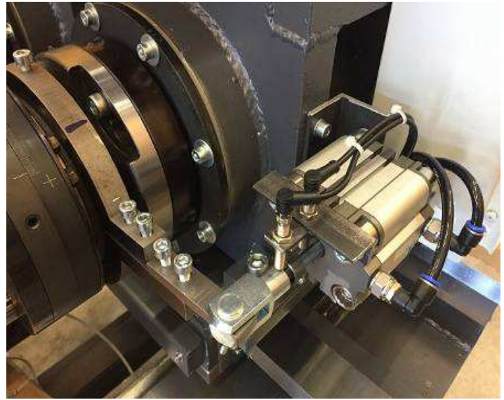
Picture 67: Standard switches, standard cylinders; easy to care for the maintenance
