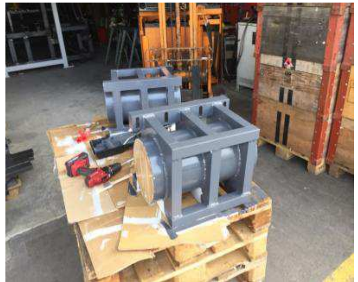
Picture 19: Paint priming and 2 K
