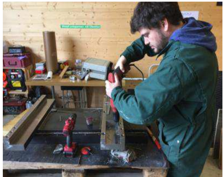
Picture 23: Drill several hundred mm lubrication channels that admission is only on one side per lane
