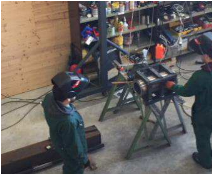
Picture 17: Jim and Sven weld the headstock housing
