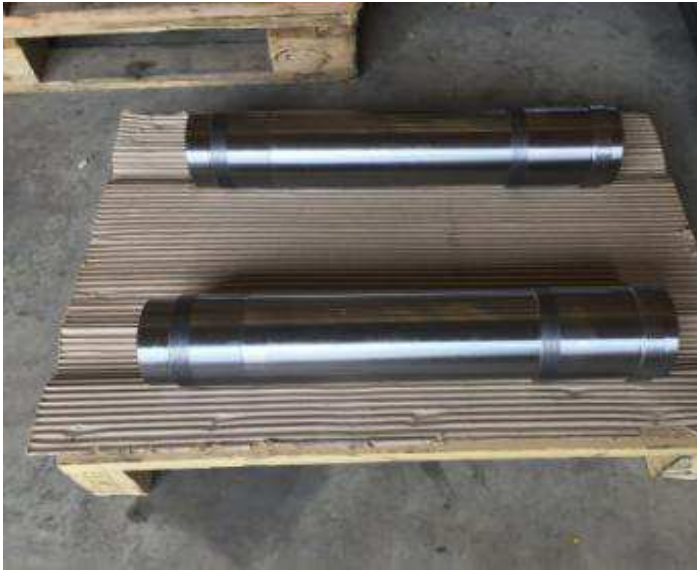
Picture 20: 2 identical spindles ground
