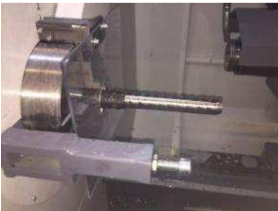
Figure 35: After peeling sees the precast, ready for rolling, like this. Diameter minimum with pitch diameter. It should be noted that parts are magnetic. From time to stay chips, hanging by the magnetism of the part. A guard covers the whole food.
