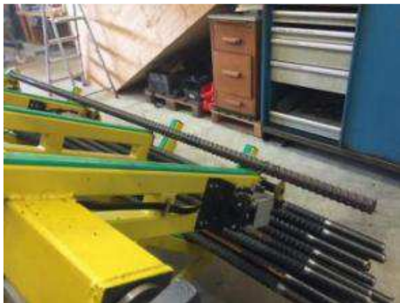
Figure 53: The prefabricated holder lowers slowly, in-cycle and opens below the claw so that the thread side falls down later.
