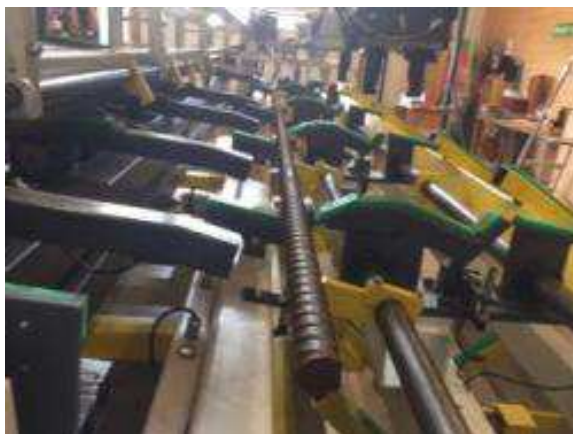
Figure 13: The blank falls on the pre-state position. Although three pieces come together, it does not bother, because the blank claw then makes the final separation. The separation is necessary so that the hook during lowering has no interference contour. Report 2 photocells workpiece in a preliminary location, position exists. The blank claw can only rotate when as both light barriers are operated.
