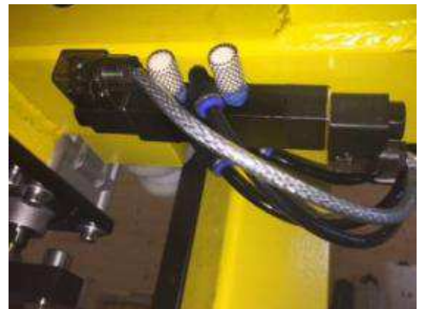
Figure 20: The valve for the movement of the bottom of the HLV. Near the cylinder, so that the movements are more dynamic.
