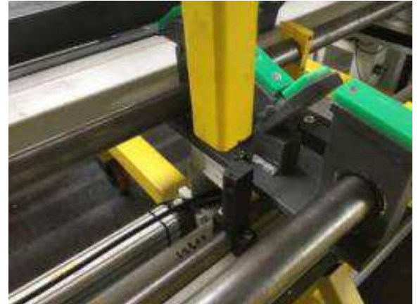
Figure 19: The pressers can solve without screw, are parked in seconds for various workpiece lengths.
