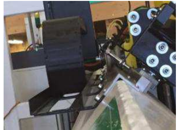
Figure 45: The racks prevents end position, that when the Y axis motor would be removed once and the machine loses the position that no unwanted is possible via the racks driving. The machine does not require a reference point more. You always know where it is, as long as the engine is not removed with the integrated measuring system without marking.
