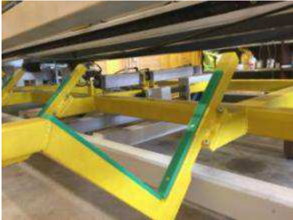
Figure 55: Cylinder 80 mm, diameter 80 push the precast car, depending on the M function in the CNC program into place.
