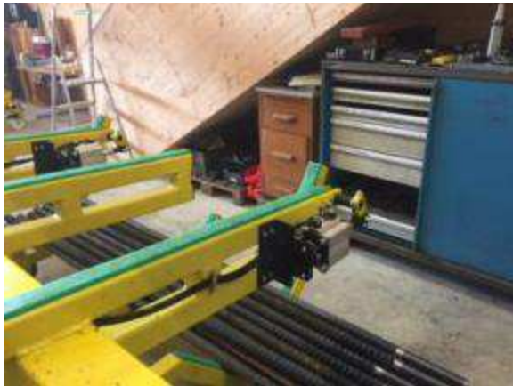
Figure 48: The finished part claw rises upward to the finished part can be intercepted, i.e. uncontrolled fall to the finished parts. The foremost cylinder, thread side, lowers delayed so that the workpiece does not fall onto the thread and being injured thereby.
