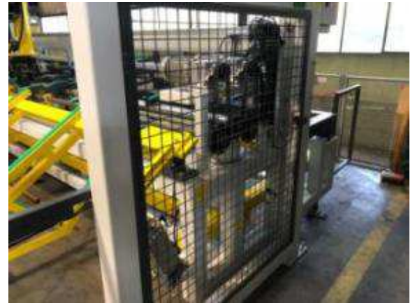
Figure 58: The whole area is protected by three guard. Screwed. Nevertheless, with light barriers. Rear view.
