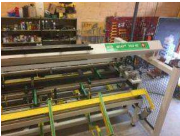
Figure 56: HLV 40 is called the auxiliary charging device 40, for 40 kg Pallet weights. The maximum length of the parts may be 4010 mm.
