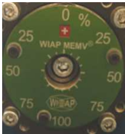
Figure 5a: The eccentric stage can be set with this scale of 0 to 100% .
