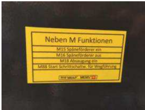
Figure 37a: The chip conveyor always only runs for a short distance, so that the chips can drain enough in slope backwards so that no water comes into the chip container. There are always dry chips in the container.
