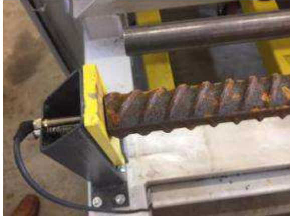
Figure 21: The switch is important for process safety. The blank can be brought to 0.1 mm into the chuck.
