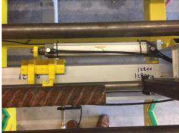
Figure 17: The workpiece pressing device which can be inverted for each rod lengths only with a handle within seconds, now pushes the workpiece forward when the two switches are operated such that a workpiece is present.
