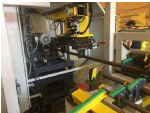
Figure 26: Here, the workpiece is driven into the machine with the HLV loader.
