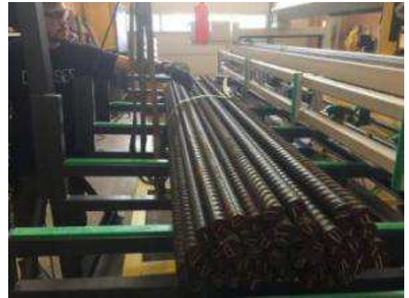
Figure 3: The federal government is cut and without manual use it distributes itself through a special vibration technology. By means of a vibrator WIAP V05 (for workpiece weighing up to 5 tons) the distribution is carried out. The vibrator can be adjustment from 0 up to 750 kg stimulator energy set.
