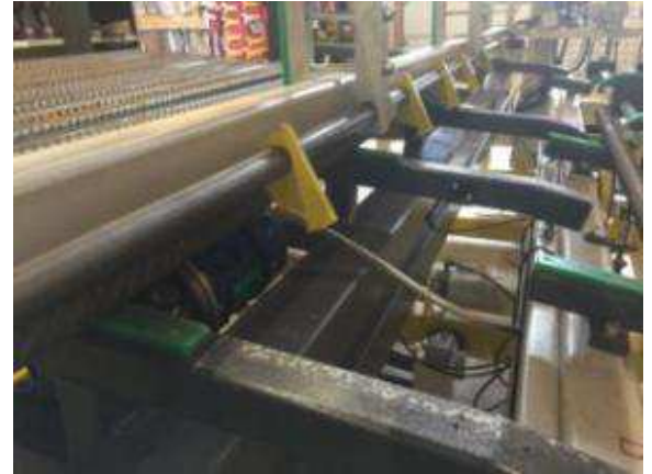
Figure 13a: Here you can see right the light barriers in the pre-state position.
