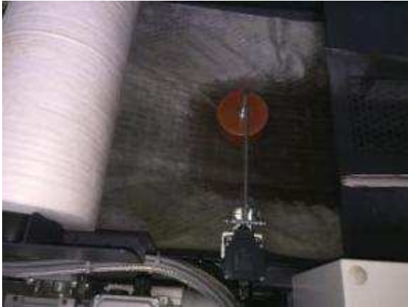
Figure 57b: If the filter is dirty, the water runs slowly and raises the switch.
