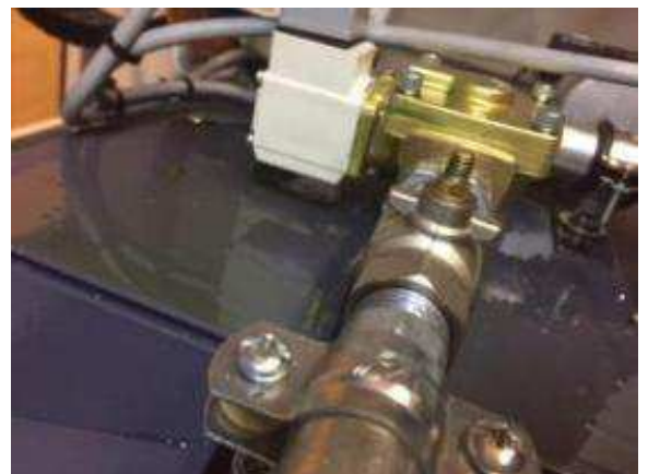
Figure 33: The amount of water can be adjusted with the tap. The water valve provides the location of the emulsion.
