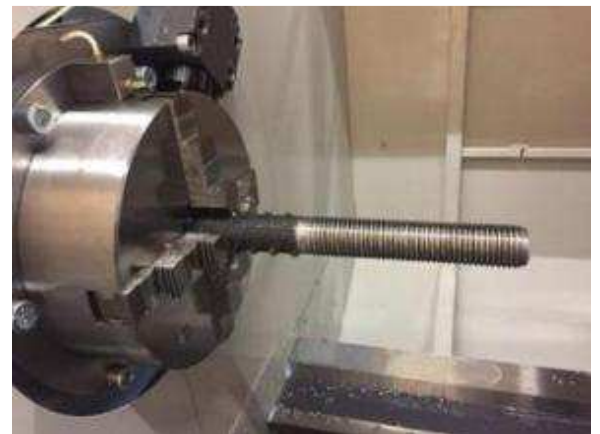
Figure 43: The finished workpiece. Here M36x4 180 mm thread length. Bake the beginning to end of thread is always 50 mm. Depending on the length of the thread everything is automatically calculated using parameters. The surgeon has no duty to enter something in the CNC program. Except: thread diameter (for the speed calculation), pitch and length of the thread and the length of the workpiece.
