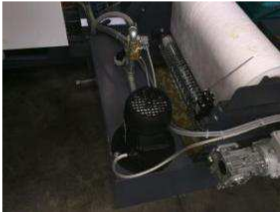
Figure 57f: In-band filter is the main pump which supplies the whole machine. If too little water will first give a warning and then the system switches to the stop mode and tells the operator what to do.
