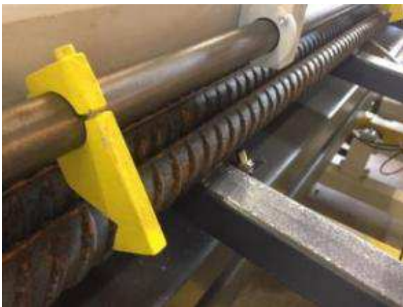
Figure 10: The blanks come slowly forward. They are held by the blank holder. Only when the two light barriers are operated, the holder can open. This prevents the parts going obliquely through the holder. It may be that more parts are used simultaneously. However, what does not bother, because the structure is designed.
