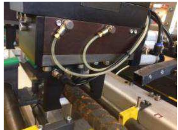
Figure 24: The WIAP grab for 40 kg include self-centering. They are monitored with 4 proximity switch. If no workpiece is present, switch the internal switch and there is an alarm. If ok, the grippers lift back to 150 mm.
