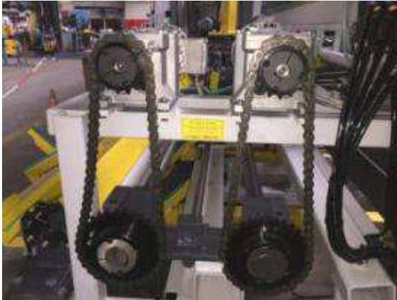
Figure 14b: The blank claw and claw finished part are driven by two central rods. The basic position is always when they are out of harm's straight down.
