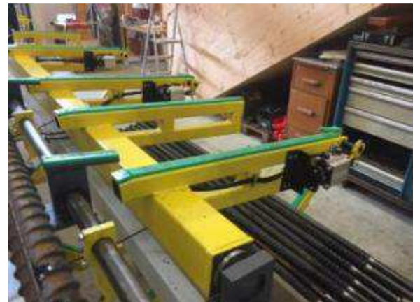
Figure 47: The filing "rake" moves up on the CNC program. In the off-time with an M function.
