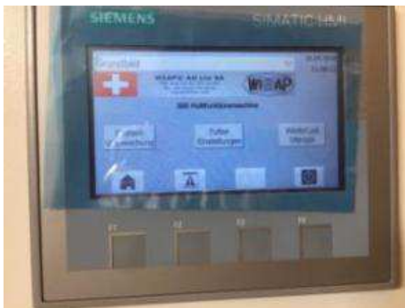
Figure 7: At the CNC control panel, side, an additional control panel. Here three operating groups for the operator can be selected. But actually, no adjustments are necessary.
