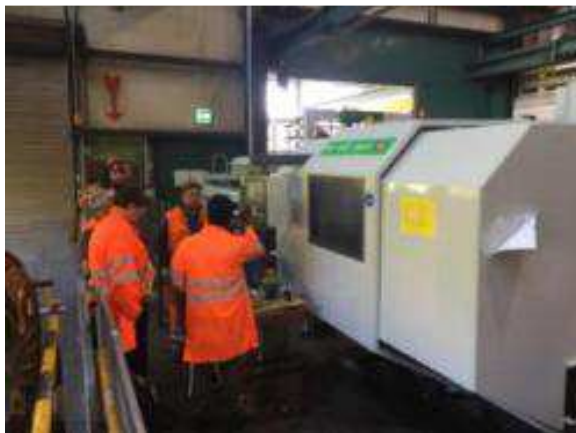
Figure 61: Timing of the machine at the customer. The plant is running with the 2.8 meters rod 12 seconds rapidly. And there is the possibility of being 30 seconds faster. But this is not necessary because the equipment is either way too fast.
