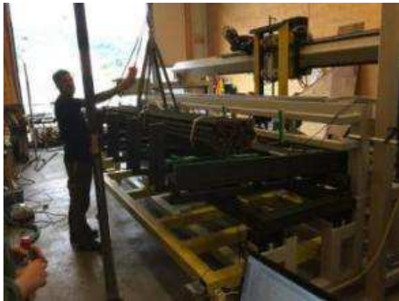
Figure 1: First, a covenant with foundation raw rods is placed on automation. 50 pieces to 2 tons. Lengths from 1.6 m to 4 meters; \varnothing 20 to 40 mm. The threads are peeled and rolled.
