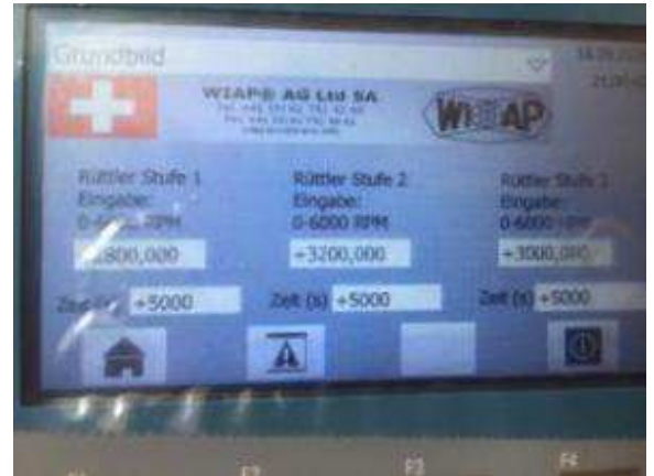
Figure 7b: The vibrator V05 can work with three speed levels. M60 stage 1, stage 2 M61 and M63 stage 3. If rods 50 are located on the automation (according piece counter), the V05 vibrates more than if only 10 bars residing on memory. The CNC program searches the zones and automatically jumps into the respective zone where M60 / M61 / M62 are selected. There is also a stepping mechanism, which switches automatically through all speeds, so even with tilted workpieces these are shaken loose.
