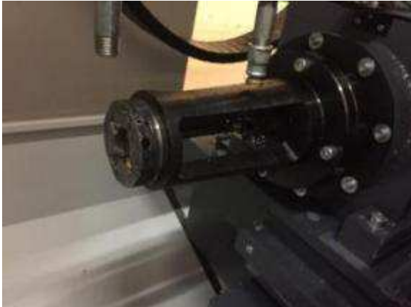
Figure 30: In the machine, the part is clamped with the chuck and then peeled with a 4-blade tool. The tool peels front with 4 plates. Each travels with 0.17 mm feed resulting 0.68 mm per revolution for four plates. Back is still a chamfering who does chamfering the inlet for the roles. He makes a 20° bevel. The chamfering must be respectively set manually for different lengths. The rotation speed is lowered and the feed rate reduced by the factor 0.6, when cutting 7 is engaged simultaneously.
