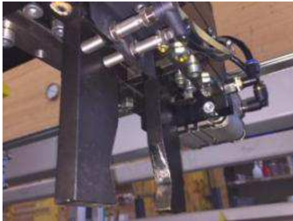
Figure 25: Gripper monitoring. Open is checked. Full interior = no workpiece or to and no switch is ok. Both gripper left and right with the same monitoring.
