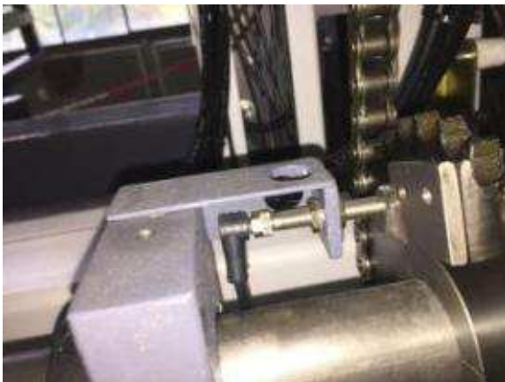
Figure 14c: A proximity switch stops the claw when it is down again.
