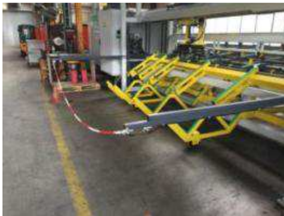
Figure 58d: The whole area is secured with horn and stop zones. The chain prevents unwitting third parties come into the danger zone. If someone runs into the stop zone, stop the whole system. There are occasionally people who get too close because they want to touch what they see.
