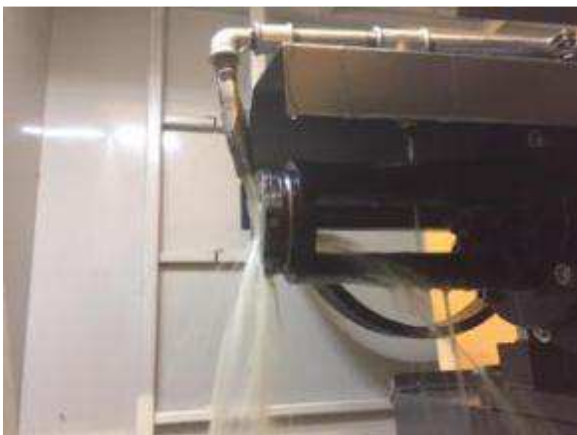
Figure 31: The peeling head is cooled with emulsion M07 peeling head, M08 burnishing head.
