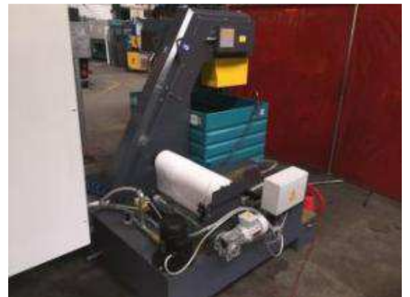
Figure 57: A band filter system ensures that the rust dust the roles of the rolling system does not prevent the long run.
