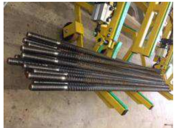
Figure 55: Finished parts thread length 180 mm M36x4. Storage for 50 pcs.
