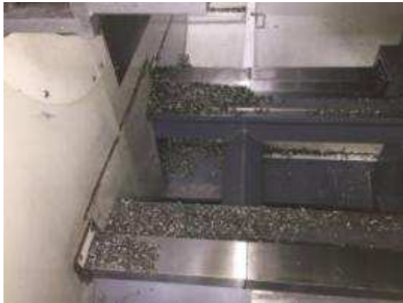
Figure 43: A function flooded the chips away; this has not been programmed here.
