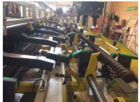
Figure 14: When the workpiece in the preliminary position is position, the blank rotates claw via an M function, the workpiece in the center position.
