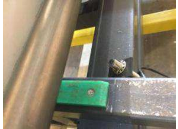
Figure 11: Monitor such 2 light barriers, whether the workpiece is present. Front 500 mm and 1500 mm. The light barriers can be set from 0 to 150 mm sensing zone.
