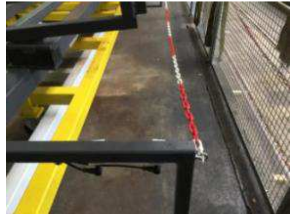
Figure 58e: Blank feeding is also controlled. First the horn zone and 150 mm progresses is shut down with stop the plant. Also here is a chain for outsiders.
