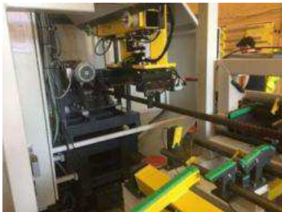
Figure 44: Then, the finished part is performed again from the machine with the HLV (auxiliary charging device). The loader lowers the part. Part removal station moves to the horizontal position.
