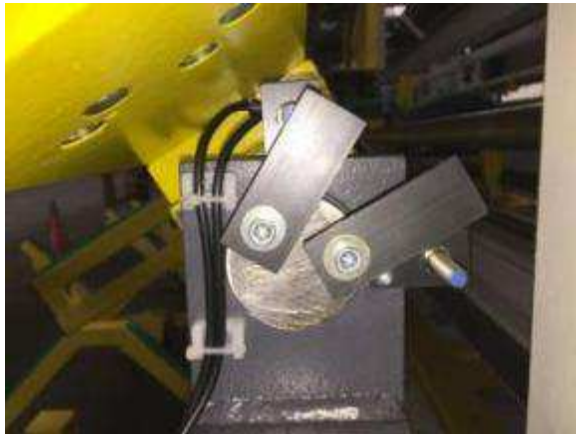
Figure 46: The location of the storage is monitored using two good adjustable limit switches.
