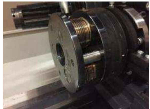
Figure 39: After peeling is rolled with the thread rolling head. The rolling head is pressed back in the lining and closed via an M function before the new rolling. Since the workpiece expands in length when rolling, we need to have the thread pitch at an increased slope of 1%.
