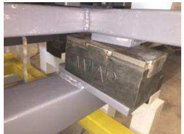
Figure 6: Several gum (100 x 120 x 200) to ensure a good damping, so that no vibrations are passed.
