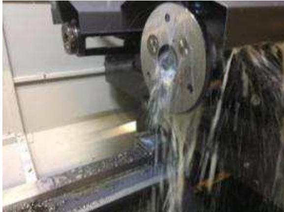
Figure 40: Also, the burnishing head is cooled with emulsion; M08 on / M09 from.
