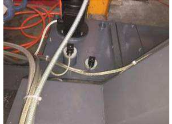
Figure 57d: The chip conveyor has a switch, level up and level down, and automatically pumps the water to the belt filter.
