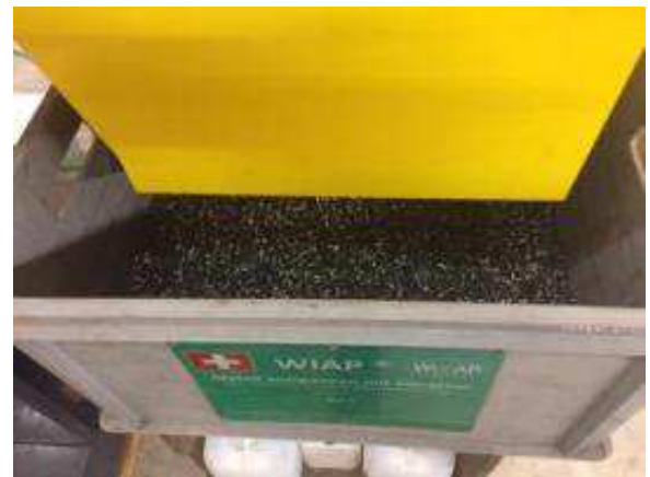
Figure 37: 100 bars give about this chips volume.
