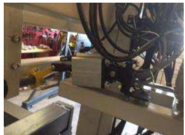
Figure 8: The blank holder with a 60's cylinder, ensures that a workpiece can migrate controlled forward.
