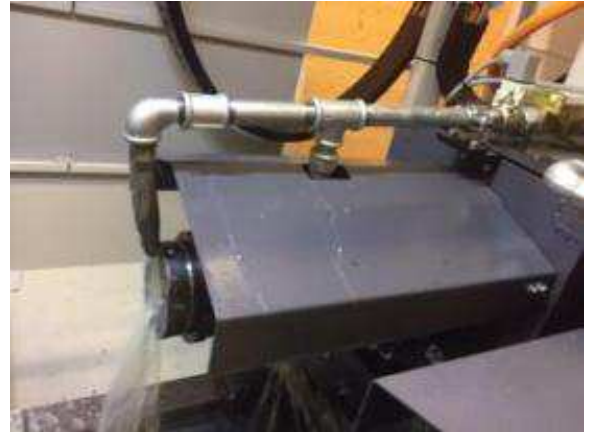
Figure 32: The guard reduces the spraying of emulsion in the engine room. Even so the engine above does not require an additional cover.
