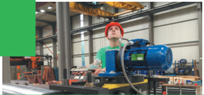
Rolls during vibration stress relief on metal (MEMV®) - Jim Peter Widmer - April 2017 (hpw)
