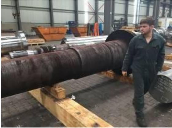
An annealed roller vibrates at a logging of differences from the non-annealed roll. The measurement is clear: an annealed roller makes no G-displacement in two axes and a 1/3 G-shift to the unannealed roller.
