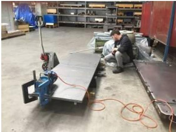
This plate was flame directed 2016 and burned. She was vibrated with 2D and 3D. The client has processed an annealed and as a comparison, a vibrating plate. Result: the annealed plate has not cleared, the relaxed vibrating plate screwed up, however, on the entire length by 0.6 mm. The customer was not satisfied, despite the fact that a plate which was not treated
