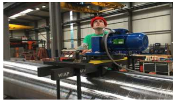
Rolling in the metal stress relief with vibration (MEMV) - Jim Peter Widmer - April 2017 (hpw)
