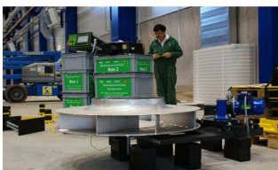
Figure 22. Impeller on a multiple-jig in Tampere, FI - August 2017 (jw)
