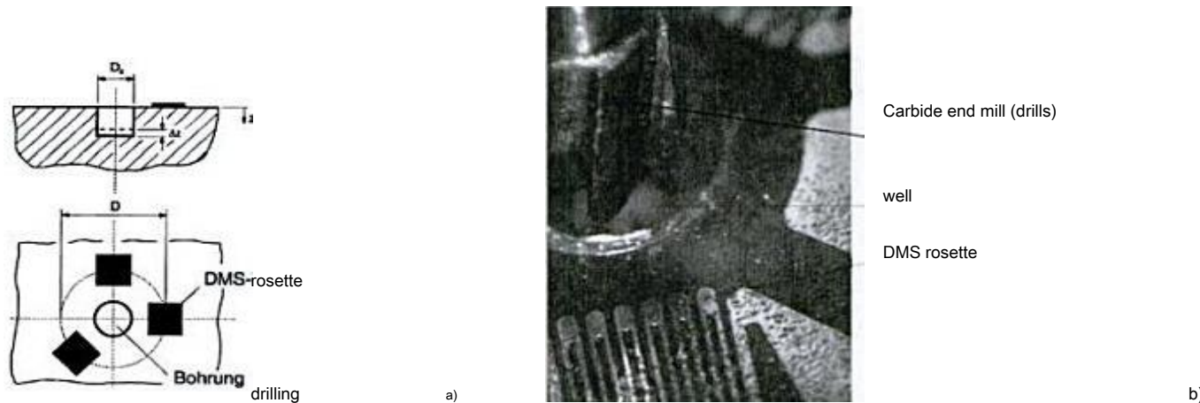
Figure 4.13: Measurement setup, the hole drilling method, diagrammatic representation metallic Observation of the drilling operation with the video microscope
