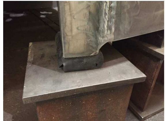
Figure 13: Here, the 60% of the rubber pinch has been reached, more should be avoided.
