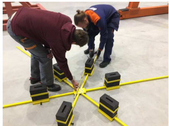
Figure 4: WIAP® MEMV® 6 star-pad- device 1300 mm diameter is set in the positions of the support. It is thus prevented that the rubber pads can migrate away at resonance movements. If need be, that the operators prevent tipping when entering the impeller. The outer diameter of the impeller was 1500 mm; the rubber has set in radius 650 mm.
