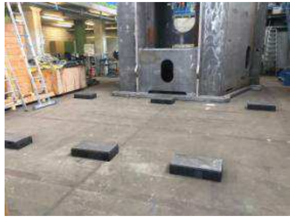
Figure 9: rubber pads for 110 tonnes: (See more Detailinformationen from the report WM877 60 tons).
