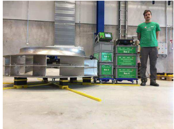
Figure 3: WIAP® MEMV® relax duplex impeller. Jim Peter Widmer fully automatic with the WIAP MEMV E control unit and printer logs measurement before and after.
