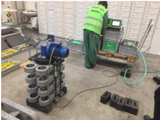
Picture: WM_865_40. Artificially aging of castings.
