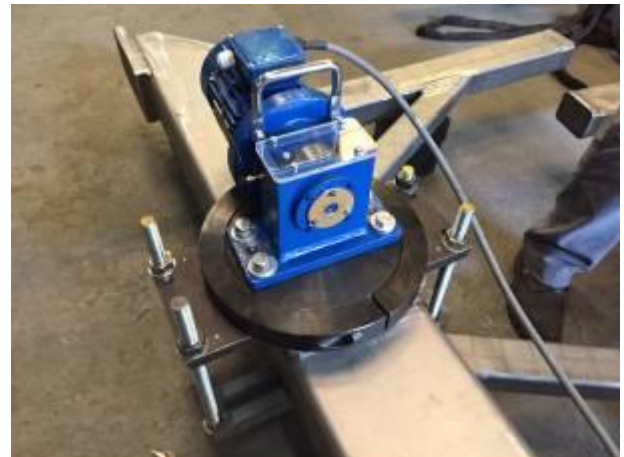
Figure 2: racks for an aircraft builder. These are treated MEMV, that vibrates. (Photo hp)
