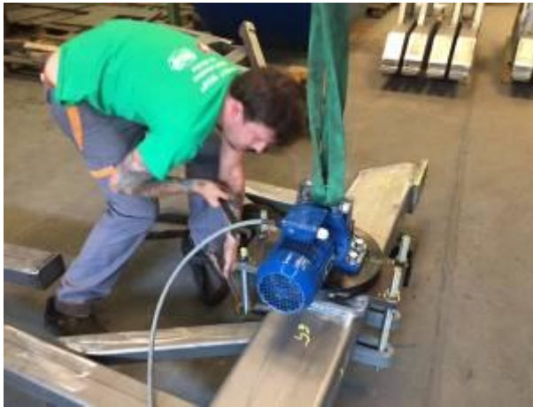
Figure 4: The good fixing is important to have the G excitation in the handle, respectively. really be able to measure. (Photo hp)
