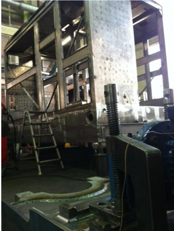
Figure 7: Here chassis MEMV be treated for one of the most powerful steam locomotives in the world. Built for Brazil. Vibration Relaxed (Photo sw)
