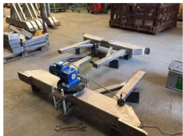
Figure 2: racks for an aircraft builder. These are treated MEMV, that vibrates. (Photo hp)
