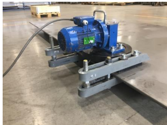
Figure 2: Test XY1 attachment of the exciter. There was the noise level to over 90db. Thinner nuts would have fixed the problem.
