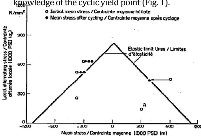
Fig. 1. Local alternating stress as a function of the mean stress
