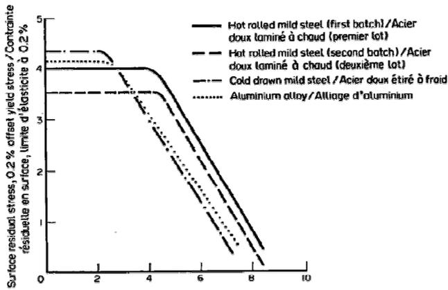
Fig. 2. Residual stress as a function of the cyclic strain amplitude
