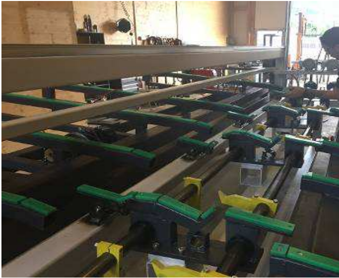
Picture 77: Wear plastic, also protects against noise
