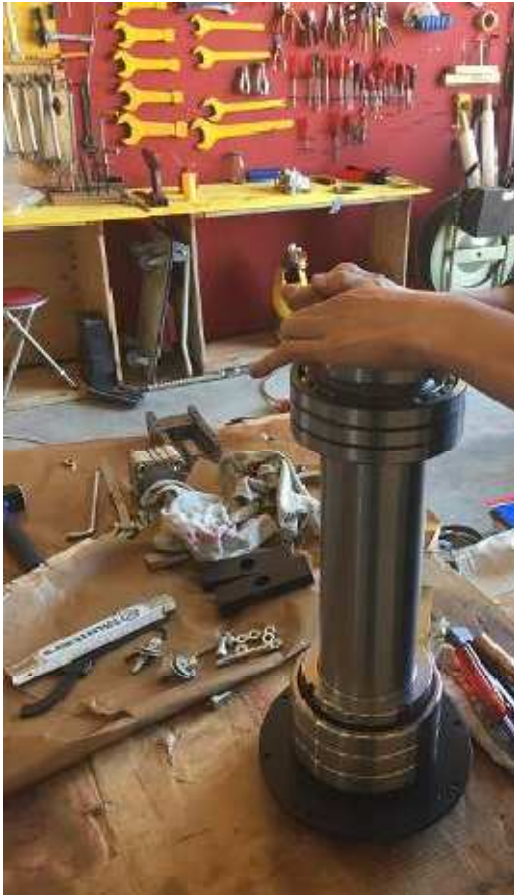
Picture 53: So now the assembly of the two main spindles
