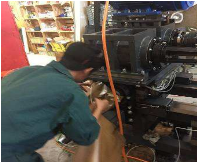
Picture 58: Installation of adjustment that the headstock can be adjusted at the hundredths. He is easy on both sides reference surfaces for spindle bore, that the belts tighten
