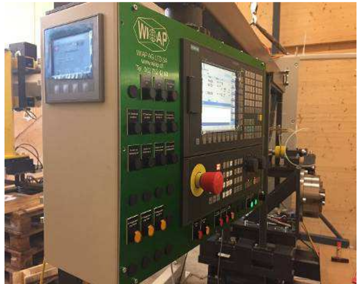
Picture 64: Since the CNC no analogues has inputs and outputs, we have taken a PLC with HMI operation. It was easier to do as a Poti solution. The tool breakage monitoring of roller burnishing tools and peeling head monitoring for all threads on M function programmable. Like the food setting with Amp. And the setting of the vibrator of the parts supply goes beyond the PLC with HMI
