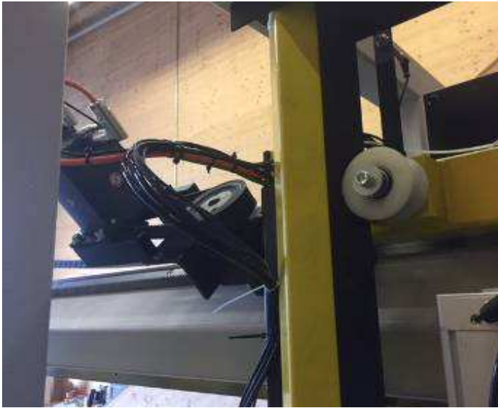
Picture 97: At 40 kg to 4 meters long stank go to a feed requires a stable solution. We have not saved with the steel weight
