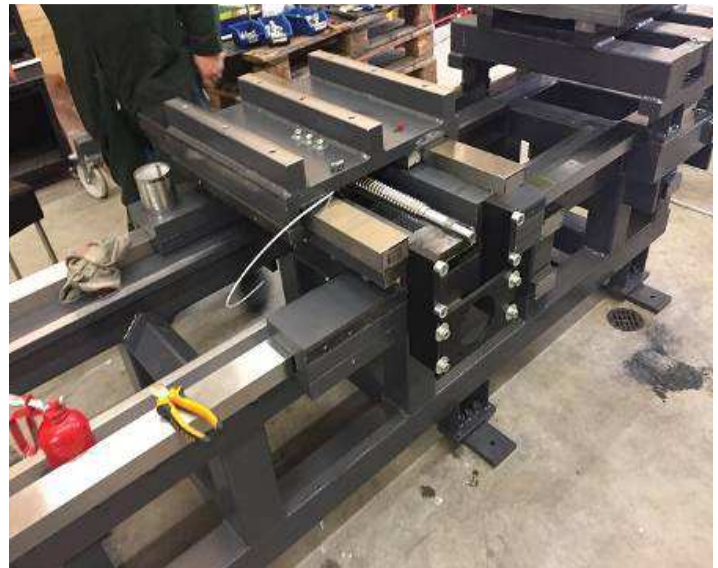
Picture 44: Cross slide in the assembly
