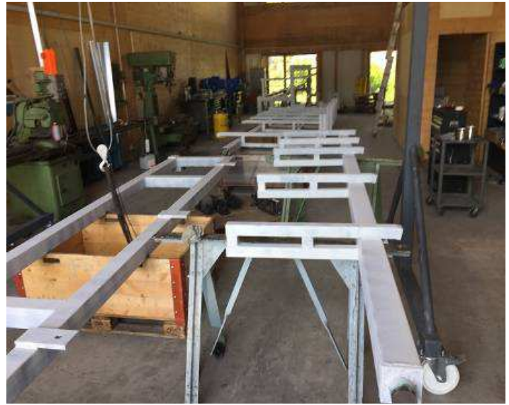
Picture 75: Everything has been primed with 2-component paint and painted
