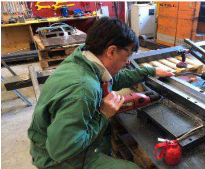
Picture 25: 150 mm deep drilling for lubrication
