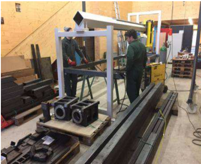
Picture 30: Welding beginning of the HLV supply and carrying away
