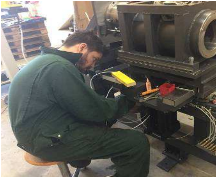
Picture 46: Sven, assembly of the lubrication
