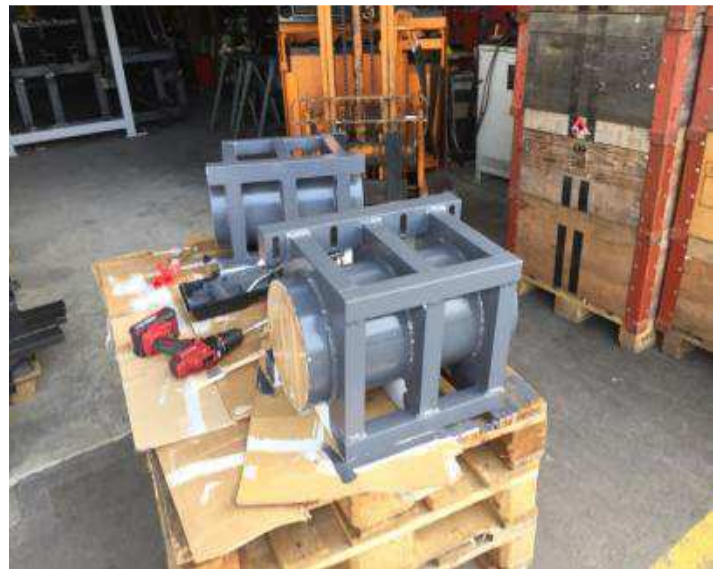
Picture 19: Paint priming and 2 K
