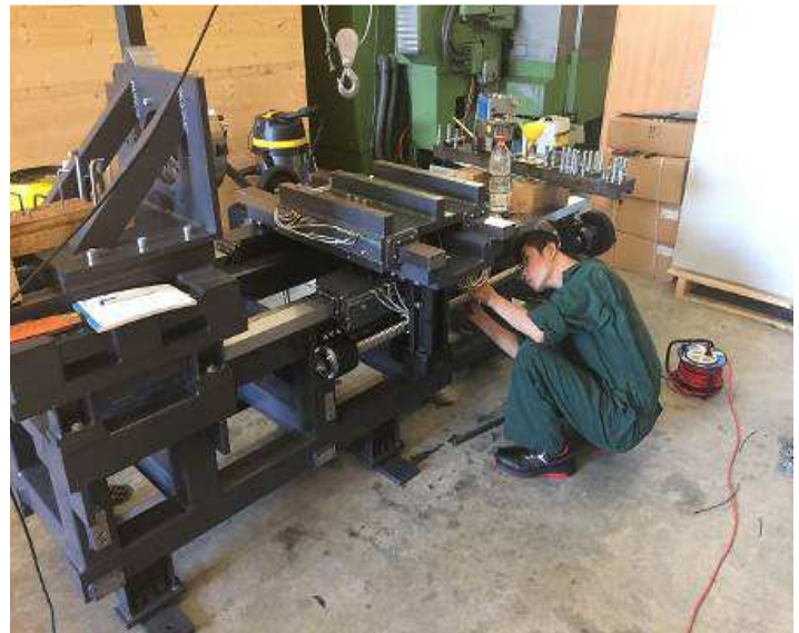
Picture 52: Ball screw lubrication and cover assembly
