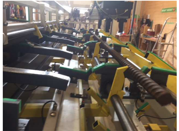
Figure 14: When the switch blank report in advance position, rotate the RP claw.
