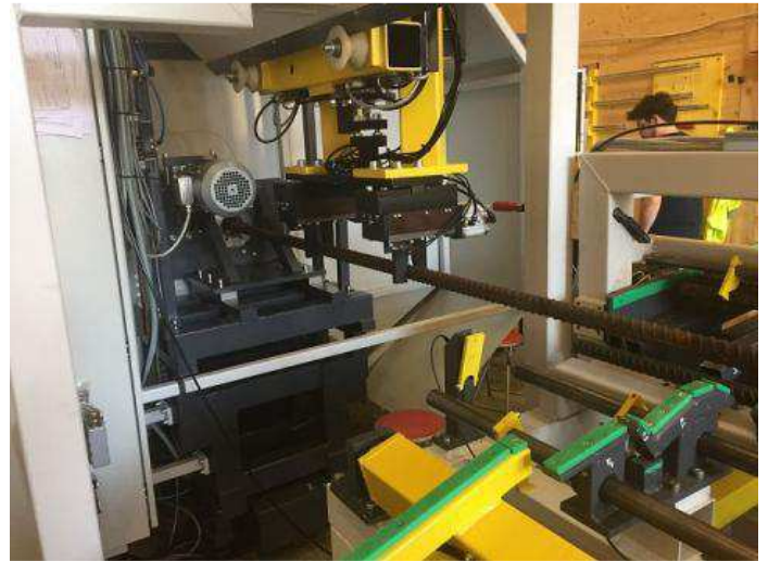
Figure 26: Here, the workpiece is moved into the machine with the HLV loader.
