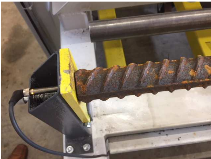
Figure 21: The switch is important for process safety. The raw part can be brought into the lining to 0.1 mm.
