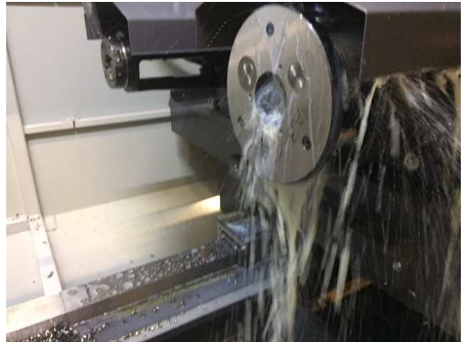
Figure 40: Also, the burnishing head is cooled with emulsion, a M08 M09 off.
