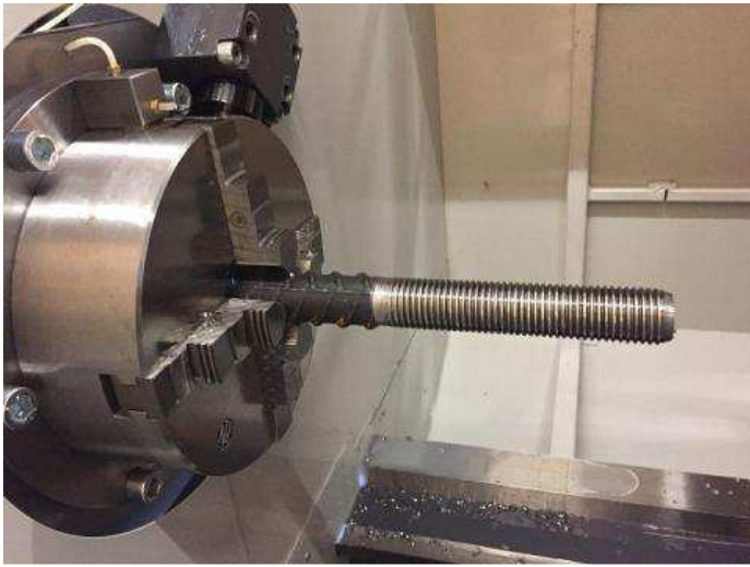
Figure 43: The finished workpiece. Here M36x4 180 mm thread length.
