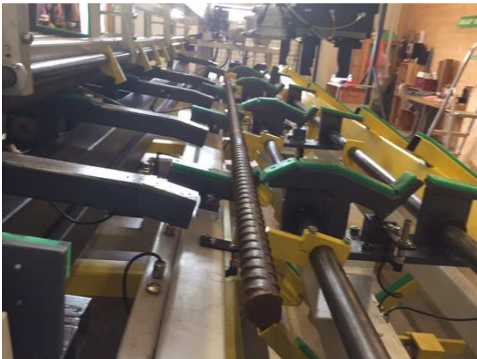
Figure 13: The blank holder opens one blank, going to the preliminary position Pos.
