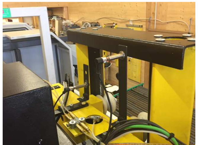
Figure 23: 2 check photocells if the grippers are up or down.
