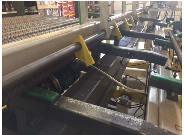
Figure 9: The blank holder waits for blanks.
