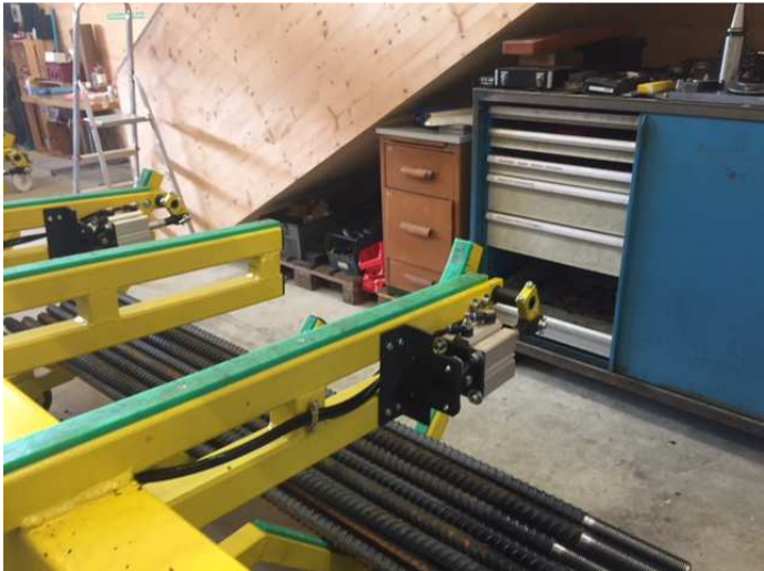
Figure 48: The finished part claw lifts upwards that the finished part can be intercepted, ie uncontrolled fall to the finished parts.
