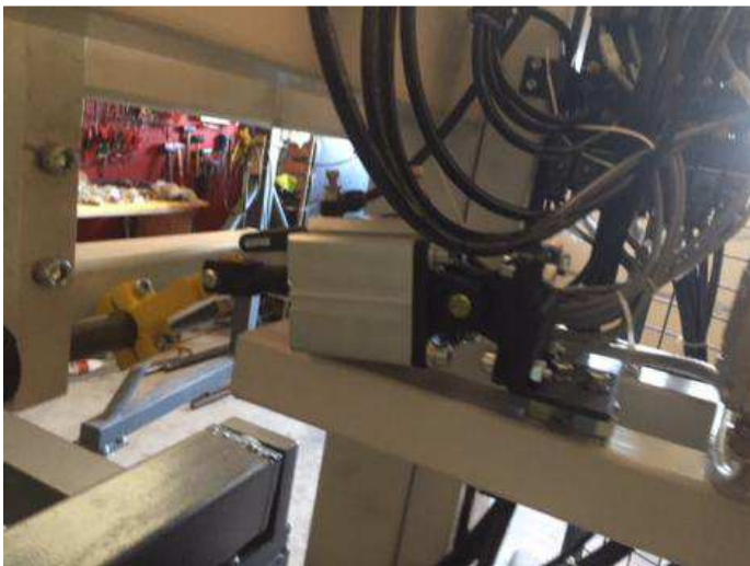
Figure 8: The blank holder ensures that a controlled workpiece forward move is possible. 2 photocells ensure that when workpieces blank press the barrier 5 seconds that the cylinder opens the blank holder. He opens up at one of the following mounted thereon light barrier, the signal is drove through workpiece. Then, this cylinder closes again. It may be that several parts are the same, but that does not bother, because the structure is designed.
