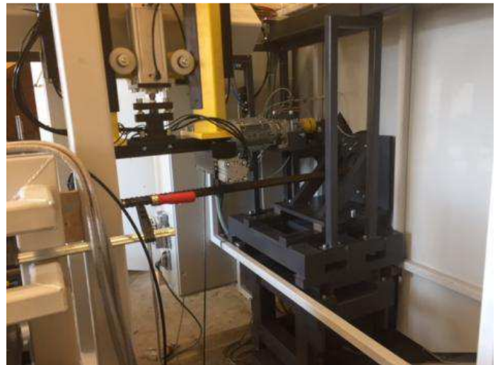
Figure 27: A chuck in the machine is a geared motor of 180 Nm reach can be closed and opened.
