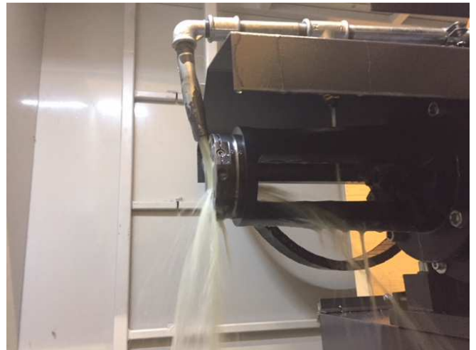
Figure 31: The peeling head is cooled with emulsion.
