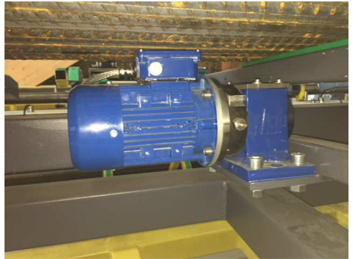
Figure 5: The vibrator WIAP V05 ensures that he can from the eccentric level 0 - 100% can be set with 2 6 mm allen keys.
