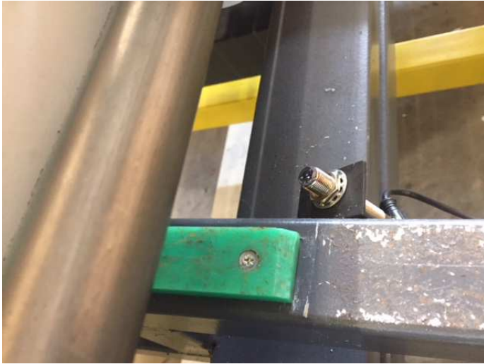
Figure 12: 2 photocells wait for the workpiece.
