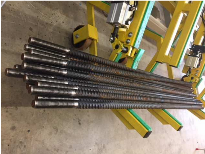
Figure 55: Finished parts thread length 180 mm M36x4.
