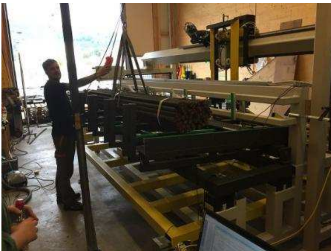
Figure 1: First, a federal foundation raw rods will put on the automation, 50 St. weight to 2 tons. For lengths from 1.6 m to 4 meters \varnothing 20 to \varnothing 40 mm.
