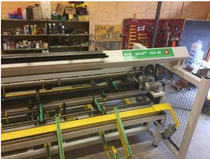
Figure 56: The HLV 40 is called the auxiliary charger 40 for 40 Kg workpiece weights. The maximum length of the parts may be 4010 mm.
