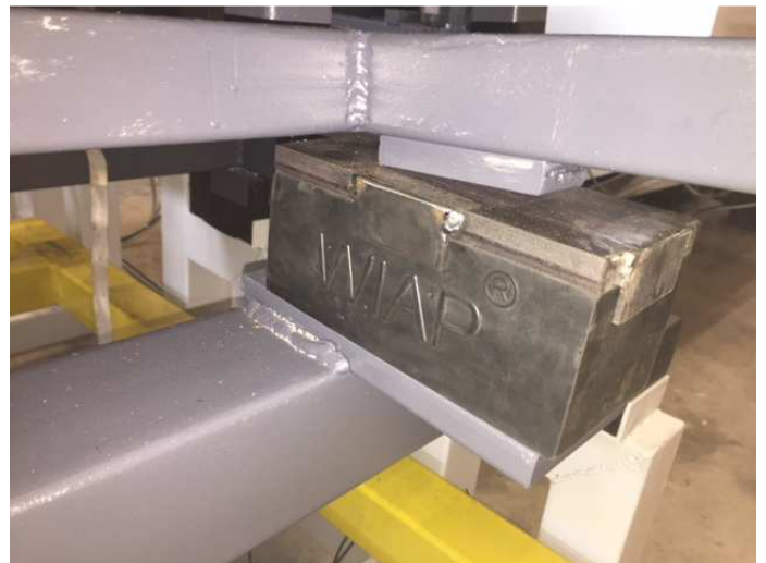
Figure 6: Several rubber provide excellent damping, that no vibrations are further provided.
