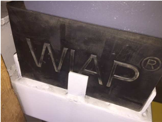
Figure 7: Thanks to the great thickness of the damping rubber is very good. The upper part vibrates, the lower part remains calm.
