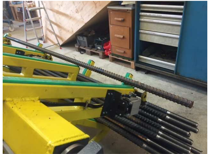
Figure 53: The prefabricated holder lowers slowly, parallel to production time And down to open the claw that the thread side from falling later.
