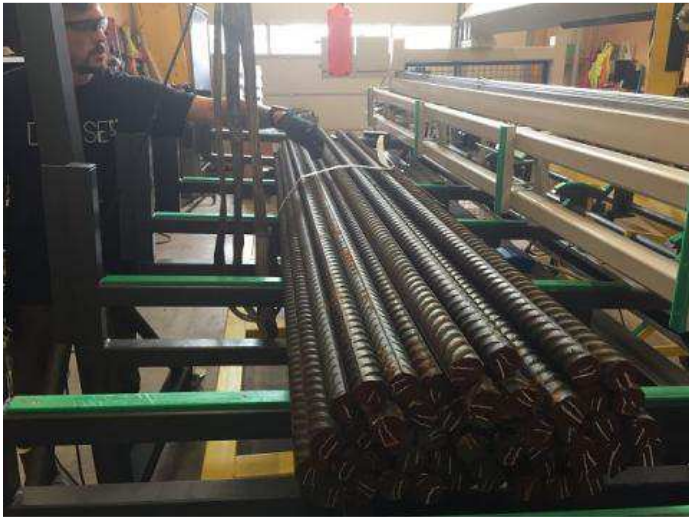
Figure 3: The collar is cut and without manual use it distributes itself through a special vibrating technique, with a WIAP for 5 tons workpiece vibrator V05, the distribution is carried out. The vibrator can be continuously adjusted from 0 up to 750 kg Stimulator energy.
