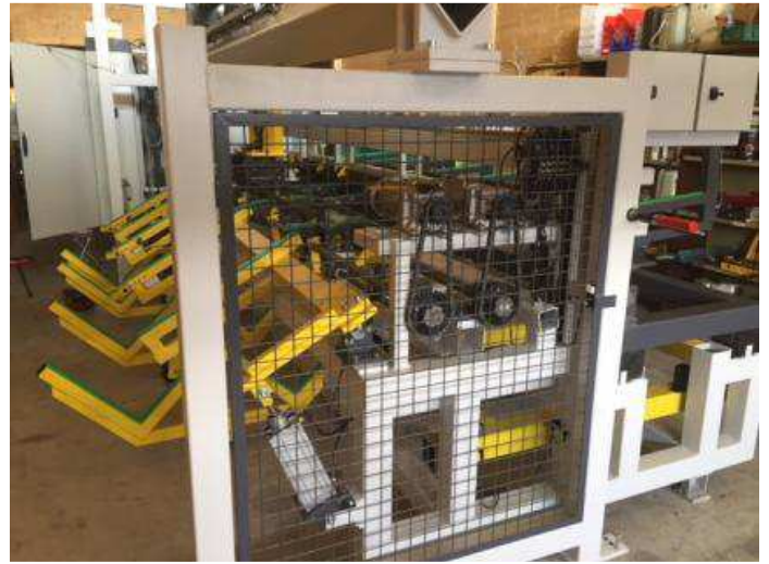
Figure 49: Then, the finished claw rotates the sprocket left under the protective grid, and places the part away on the finished part deposit, which must be available for these tasks above.
