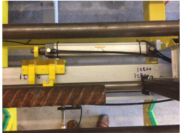
Figure 18: The workpiece pressing device now moves the workpiece forward.
