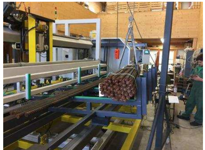
Figure 2: Just a few \varnothing 40 x 2.8-meter-long rods are ahead in the bunker, the new covenant is \varnothing 40 x 2200 still bound behind.
