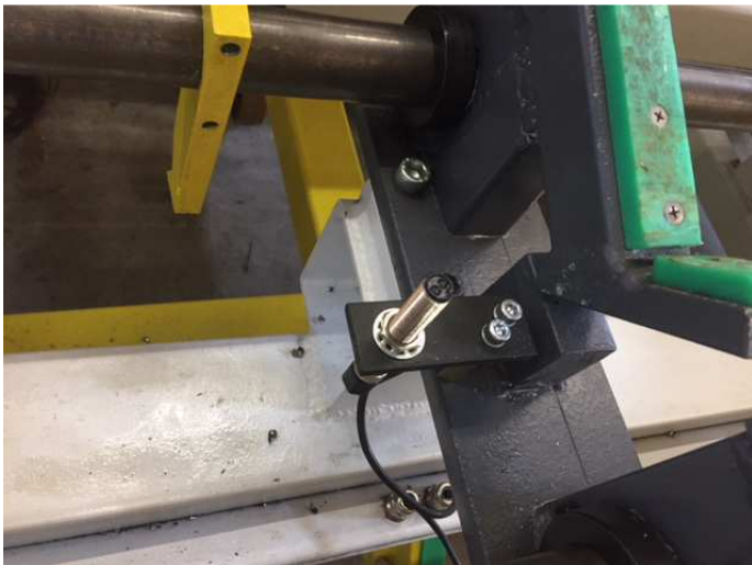
Figure 17: Checks the second light barrier, if only one photocell is there, the work piece is inclined on the support and handling should stop.
