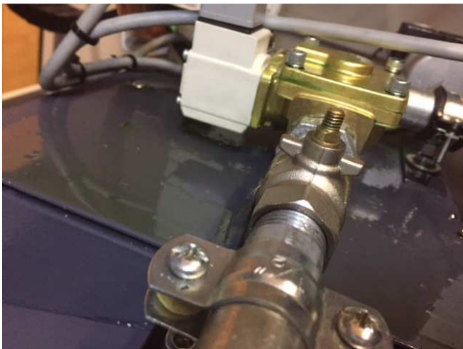
Figure 33: The amount of water can with the tap be adjusted.
