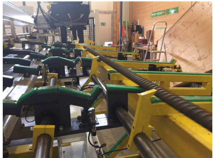
Figure 50: The finished part is lifted with the rotary claws.
