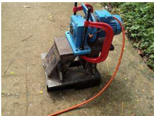
Photo 17: We do it outside because the hall floor is not good enough. The hall floor is vibrating excessively. 30 minutes at 4300 rpm is relaxed.
